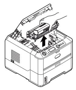
**3.** Put the assembly down gently onto a piece of paper to prevent toner from marking your furniture and to avoid damaging the green drum surface.
